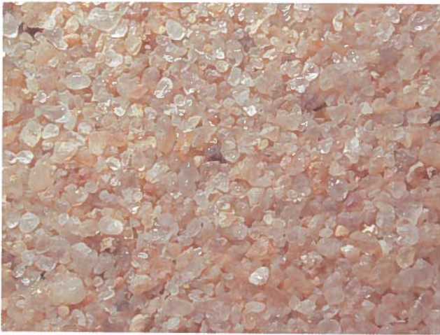
This sand from a dune in Israel could become a sandstone if a matrix glued the grains together. This image is magnified 10 times.
